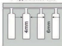
细齿型出线孔尺寸 T-Type slotted size
